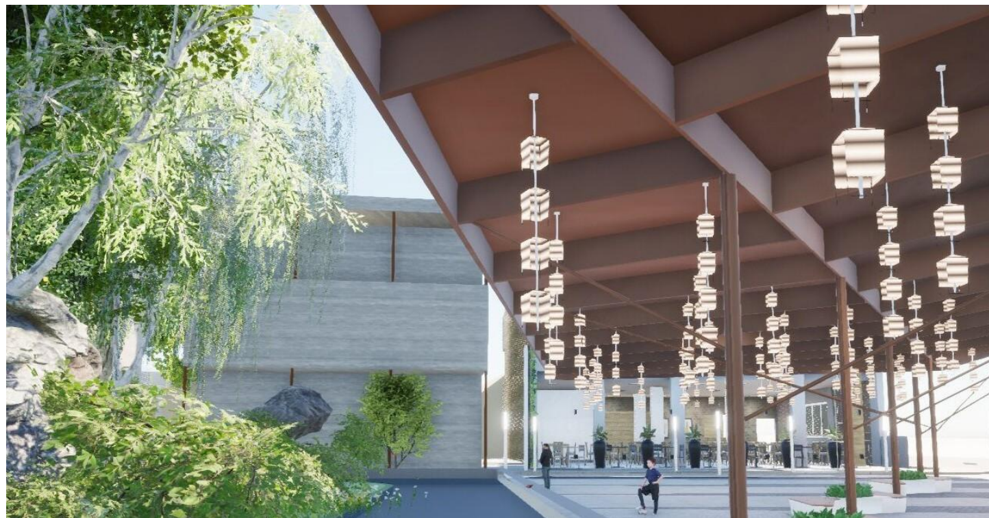
Fig. 18. Northeast perspective of the public pavillion. The centre landscape creates an opportunity for access to water while acting as an ecological spatial separation between the private residences and the main public space under the canopy. The sloped roof allows for rainwater to be directed to the water feature.
